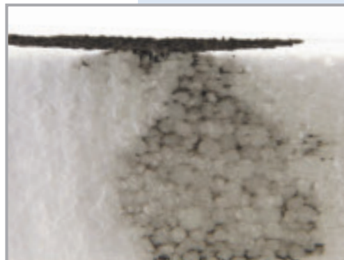
White Bead Board (EPS) Allows Moisture Migration
