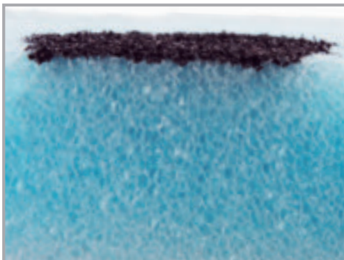
BLUE™ STYROFOAM™ Brand XPS Resists Moisture Penetration
